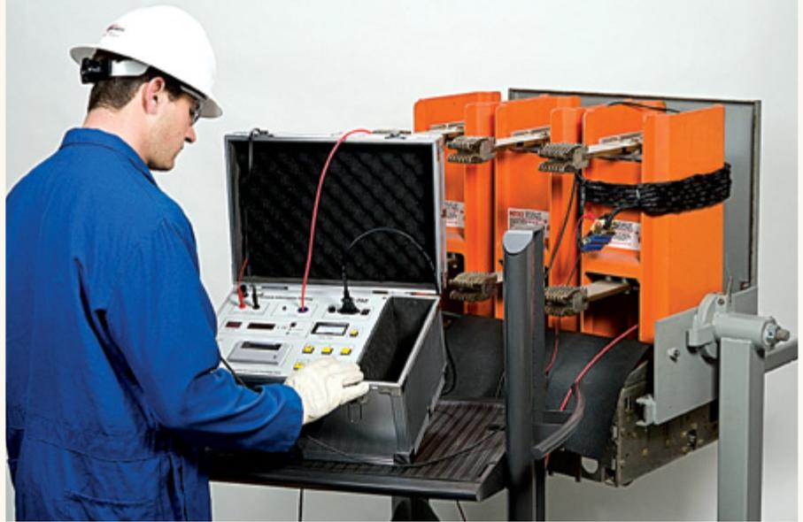
VACUUM INTERRUPTERS, INC. is proud to announce the availability of their new magnetron atmospheric condition (MAC) field and shop testing system for quantifying the remaining life of vacuum interrupters used in medium-voltage circuit protection devices.
