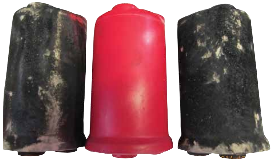
Another view of Glastic insulator bushings with flashover damage.
