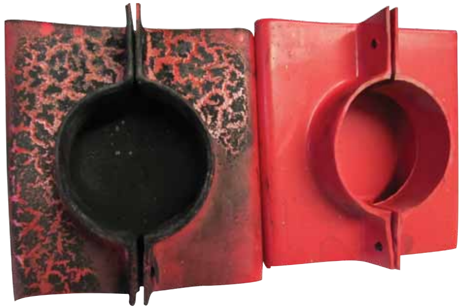
Left bus joint boot shows flashover damage from lack of regular maintenance.
