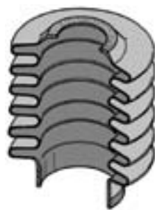
Figure 1: Cutaway drawing of vacuum interrupter bellows
