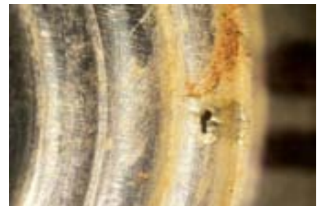
Figure 2: Galvanic corrosion in stainless steel bellows
