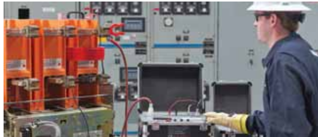
Vacuum Interrupters’ new rigid magnetic coil for GE PowerVac circuit breakers ships with an external power amplifier to boost the magnetic field strength, enabling the system to predict remaining lifetimes for vacuum interrupters installed in PowerVac circuit breakers without disassembling the OCPD.
