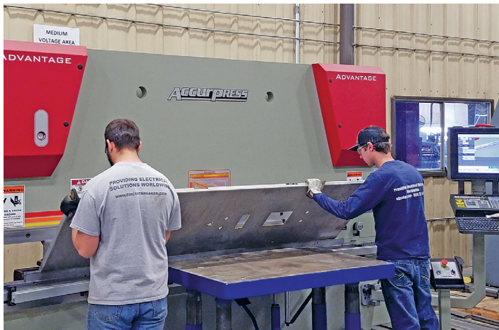
A press brake (left) and new mills (right) assure precision and easier operation in the machining of breaker and other electrical equipment components.
