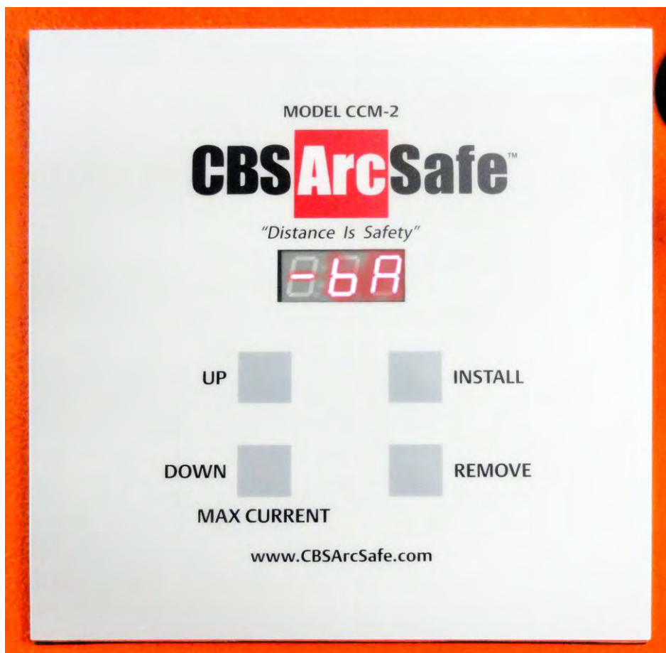
Figure 2-2: Low Battery Alert on CCM
