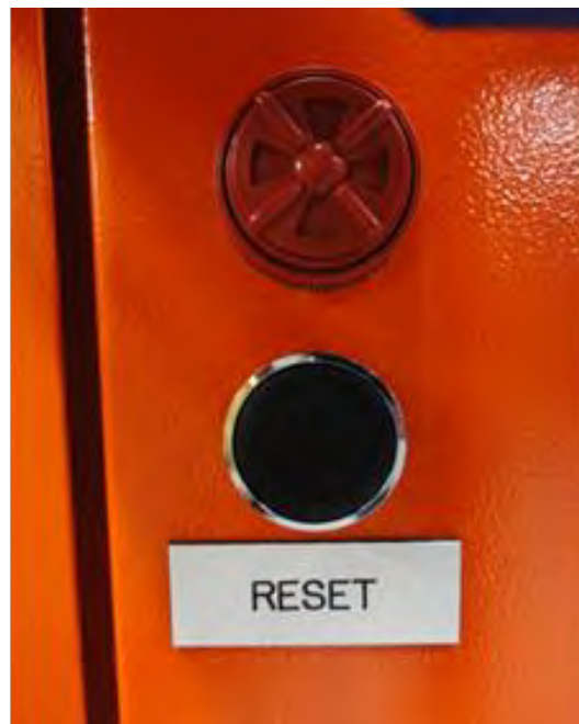
Figure 3-6: CCM Status Indicator audible alarm
