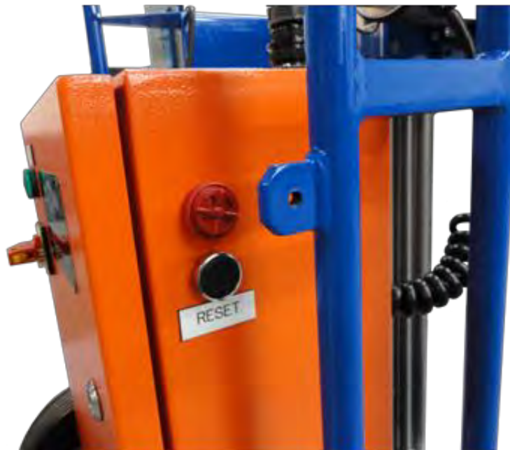
Figure 1-21: CCM Status Indicator Siren
