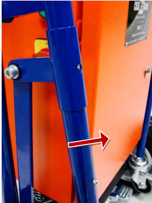
Figure J-2: Deploying the Transport Assist leg
