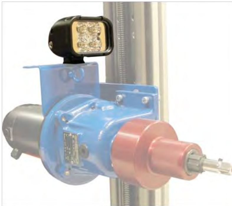
Figure E-1: LED Light installed on RRS-1
