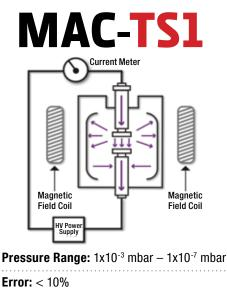
Vacuum Interrupter Test Principle: Penning Discharge Magnetron
